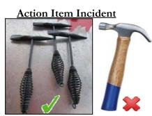
On the 19th April 2013, a LCQ mechanic sustained a 1cm laceration of left index finger due to the hammer head of the wooden hammer being loose, hence causing the finger injury. The lesson learnt from this injury is to phase out the wooden hammers and replace it with certified metal or silicon hammers.
